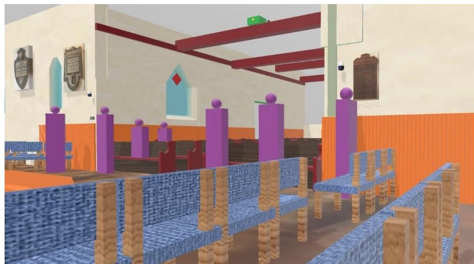
4 Impression of both PTZ cameras mounted at the corners of the North and South Transepts, together with projector mounted on forward beam in nave. Fixed camera is shown adjacent to projector, but barely visible at this distance.
